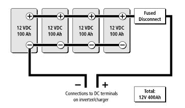
Figure 11 Batteries Connected in Parallel
